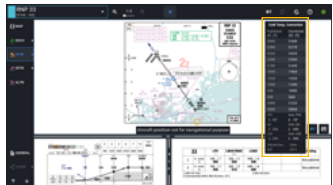
Figure 2: Cold Temperature Correction Calculator on Lido eRoute Manual
